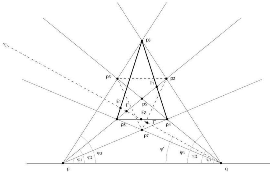
FIGURE 3. Method of Obtaining Boundary Points of the Shadow Body [4]
